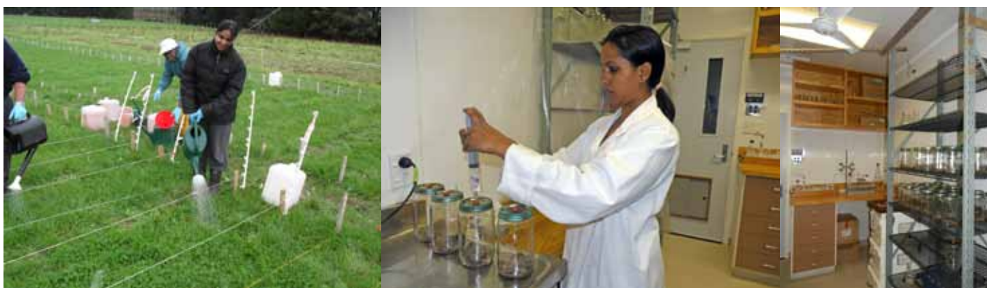
Left: Neha Jha PhD student supported by Dr Edith Khaembah (Massey University) applying cattle urine treatments to field plots at Massey University Dairy Farm-4. Middle: Neha Jha collecting gas samples from Agee-jars for measuring soil denitrification rate at Landcare Research. Right: Soil samples treated with and without urine are incubated in Agee-jars in constant temperature room
