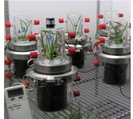
N 2 O emission measurement units in a climate controlled plant growth cabinet
